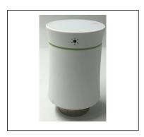
Smart radiator thermostatic head THZ controls heat output of one heating device: radiator or convector. It is installed on the thermostatic valve of heating device. There are adaptors for most common thermostatic valves in standard set.
