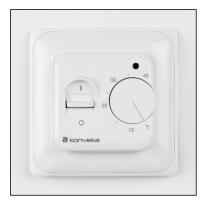
MT230 is designed to regulate the room temperature by controlling electric or hydronic underfloor heating devices. The thermostat is controlled by turning the wheel. The LED indicator shows the activity status of the heating system.
