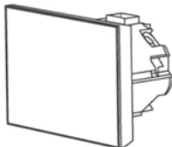
3. Place the front panel of the thermostat against the housing and press it down
