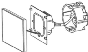
1. Connect power supply and control wires
