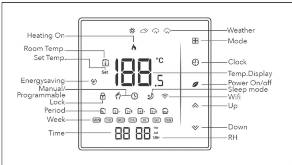
**1. Power on/off.** Press to turn thermostat on/off.
